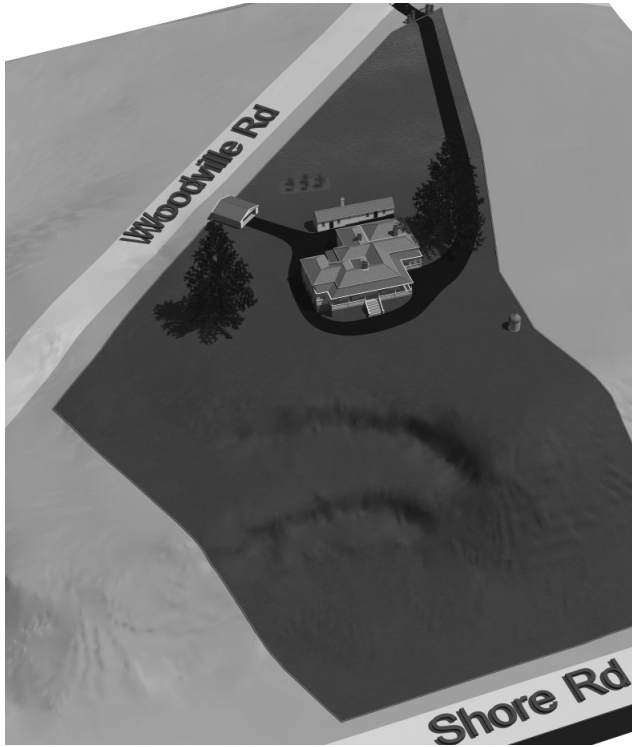
Figure 10. 3D Computer based model using LIDAR data showing reconstructed terraces.
